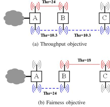
Fig. 2. Channel assignment for a linear network with three mesh nodes and one gateway. The distance between A-B is 150 m and B-C is 230 m. The transmission range is  $\approx 360$  m. Channels considered: 1-7
