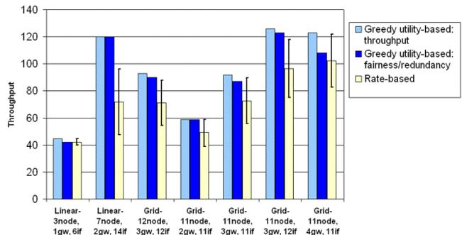
Fig. 6. Aggregate throughput achieved by the greedy utility-based and rate-based channel assignment procedures; for the latter, the average of 100 runs and the 95% confidence interval is shown. The channel assignment and node connectivity for the greedy utility-based selection procedure are shown in Figures 2, 3, 4, 5(a), 5(b), 5(c), 5(d).
