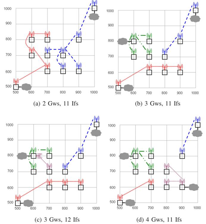
Fig. 5. Channel assignment and node connectivity for 11-node grid network. Channels: 1, 4, 7, 10. Fairness objective. (Gws: Gateways, Ifs: Interfaces)
