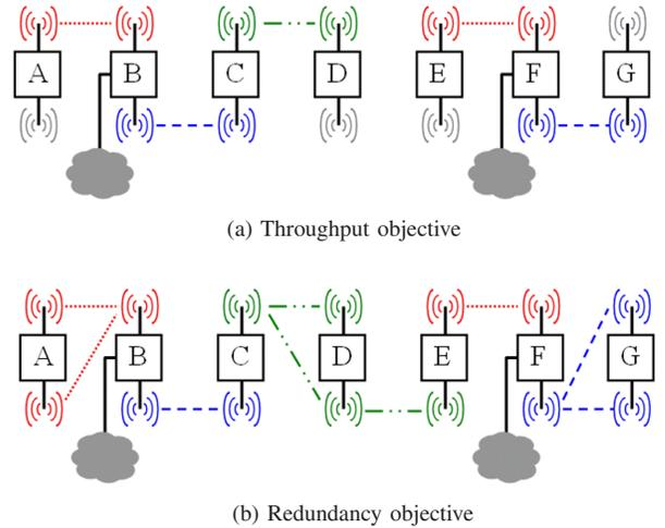
Fig. 3. Channel assignment for a linear network with 7 nodes and 2 gateways. Distance between neighboring nodes is 150 m. Channels considered: 1-7.
