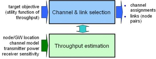
Fig. 1. The channel assignment procedure consists of two modules: the throughput estimation module, and the channel and link selection module.
