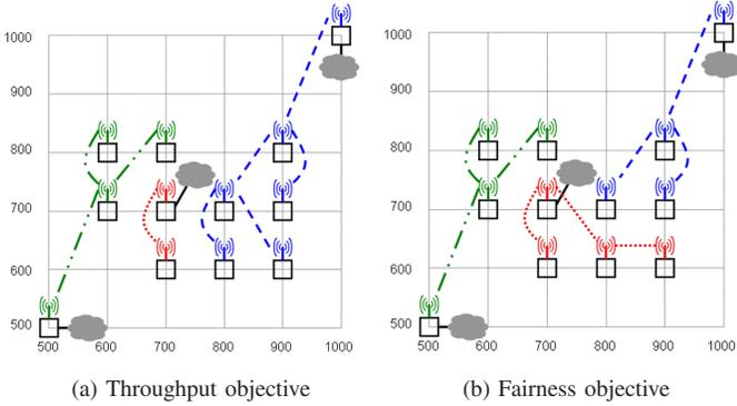
Fig. 4. Influence of target objective on channel assignment and topology for 12-node grid network. Channels considered: 1, 4, 7.
