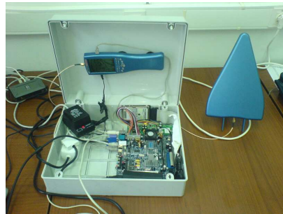
Figure 4: The EMF monitoring node contains a mini-ITX and a low cost EMF monitor (Spectran 60X0 analyzer, which can measure up to 7 GHz).
