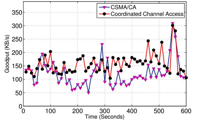
Figure 6. Aggregate Goodput of a 4 APs WLAN of 75 Users with Realistic Traffic
