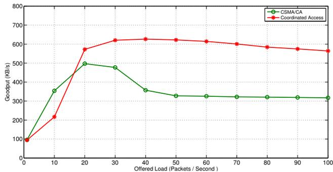
Figure 4. Aggregate Goodput experienced by all users with CSMA/CA and with coordinated access for different load levels.
